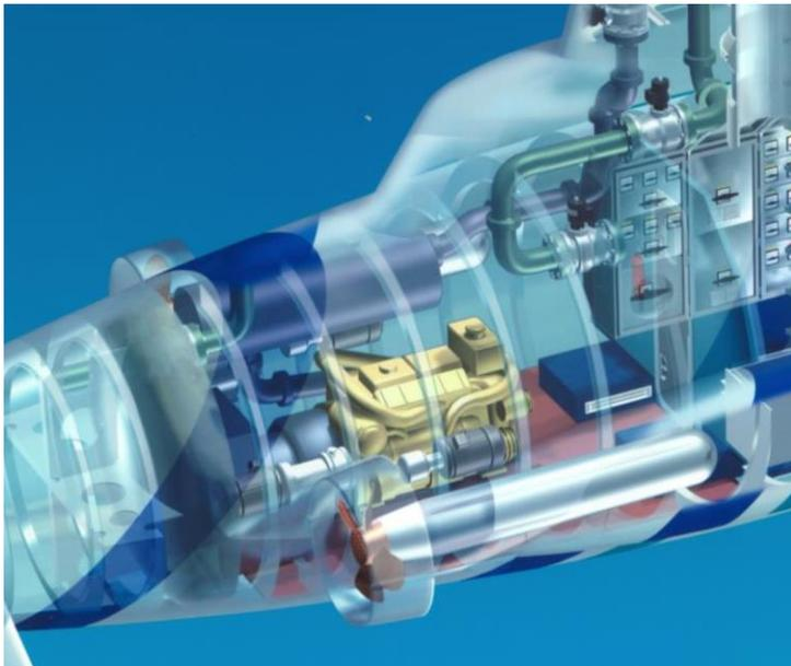
Snorkelling is made possible by a dry snorkel induction system, which allows diesel starting as soon as the induction valve breaks the surface. No time is lost in the otherwise obligatory draining. The induction mast is telescopic, in contrast to the snorkel exhaust mast, which is just the vertical end-part of the exhaust system located in the sail.
